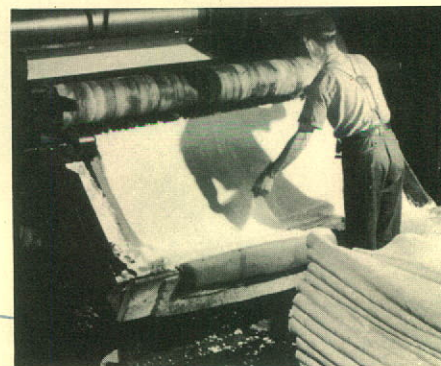
The final product—pure bleached pulp for the papermaking process
