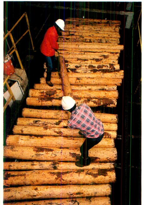
Log processing center at Holden, Louisiana, captures the residuals from lumber production to supply fiber and fuel for nearby Crown Zellerbach "core" mills.
