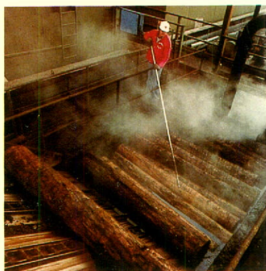
Top: Soaking logs in hot water ensures more efficient peeling at our Kelowna plywood plant.
