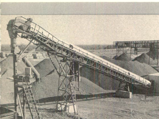
Forano Prefabricated Belt Conveyors handling aggregate.
