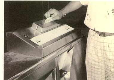
The magnetic pass readers installed in 16 stations at the end of the year improve access to the metro and simplify fare collection.
