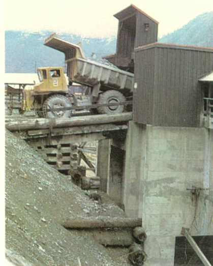
Truck dumping ore from Myra mine into storage and crushing area to begin the milling process.
