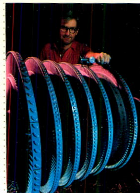
Typical steam turbine rotor assembly. The Company manufactures steam turbines in ratings up to 60 megawatts.
