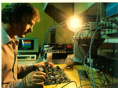
Prototype circuit boards for the SCIEX ELAN system go through performance evaluation.
