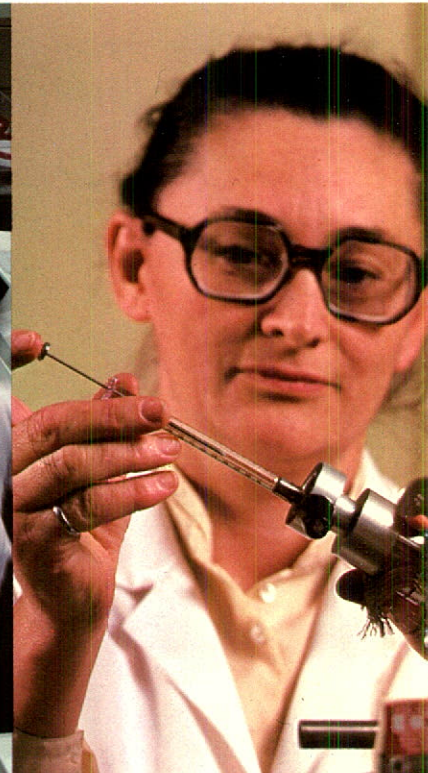
Seconds after injecting an industrial sample a readout in parts per trillion of Dioxin is obtained by TAGA ® technology.
