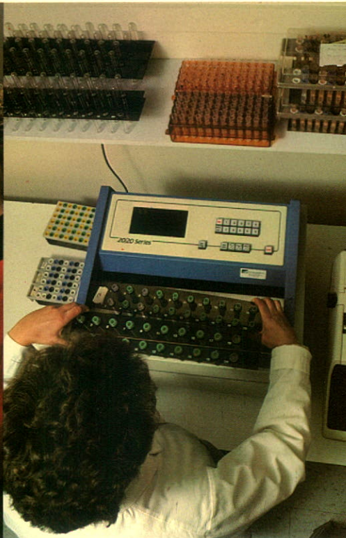
In a matter of minutes hundreds of blood samples can be assayed for constituents such as Vitamin B 12 by a high speed automatic gamma counter.
