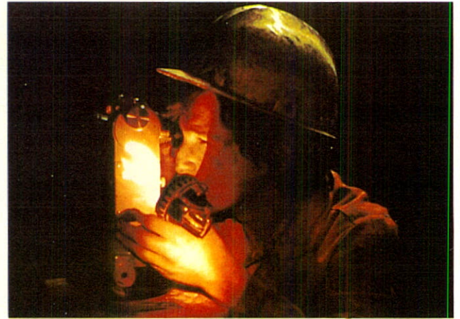
Underground mine surveyor laying out development roadway. Facing Page: Loading waste at No. 9 surface mine.
