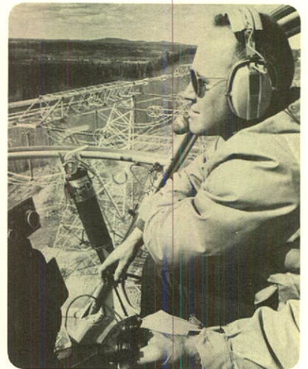
Helicopter-borne patrolman checks 500 kv transmission line from the Peace River.
