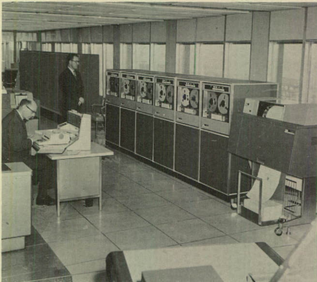
Operator's console, magnetic tape units and high speed printer - part of new electronic data processing system.
