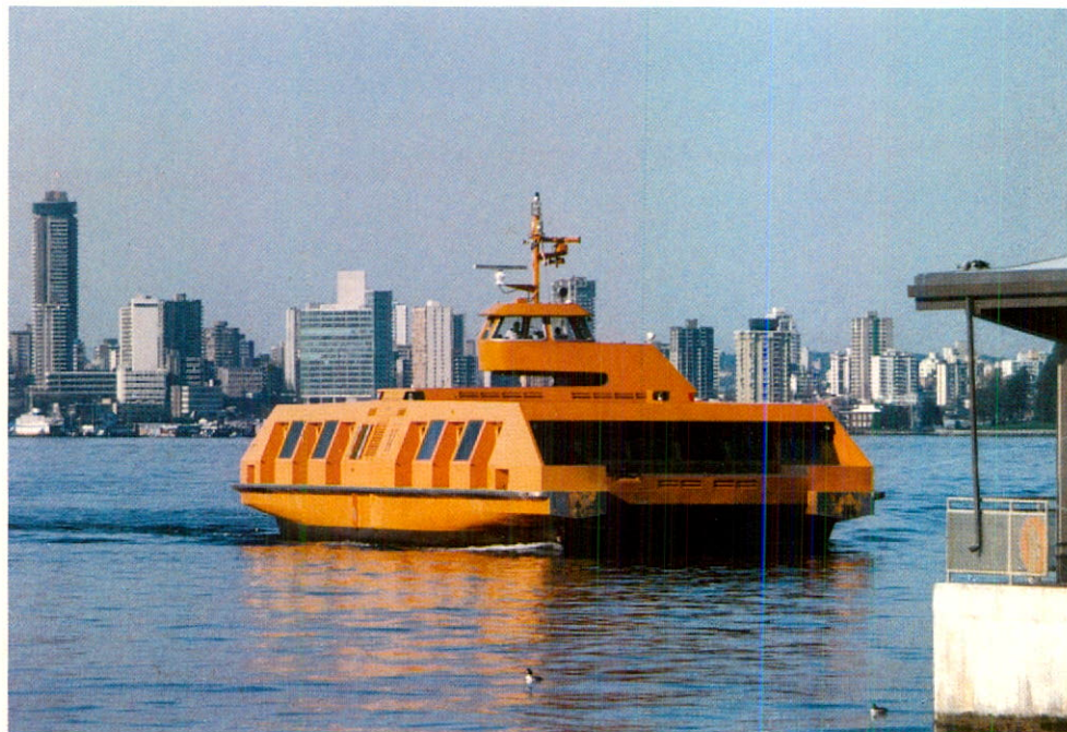
SeaBus ferry link between north shore of Burrard Inlet and downtown Vancouver was inaugurated on 17 June 1977. Two ferries of unique catamaran design had carried more than 2,700,000 passengers by the end of the fiscal year.
