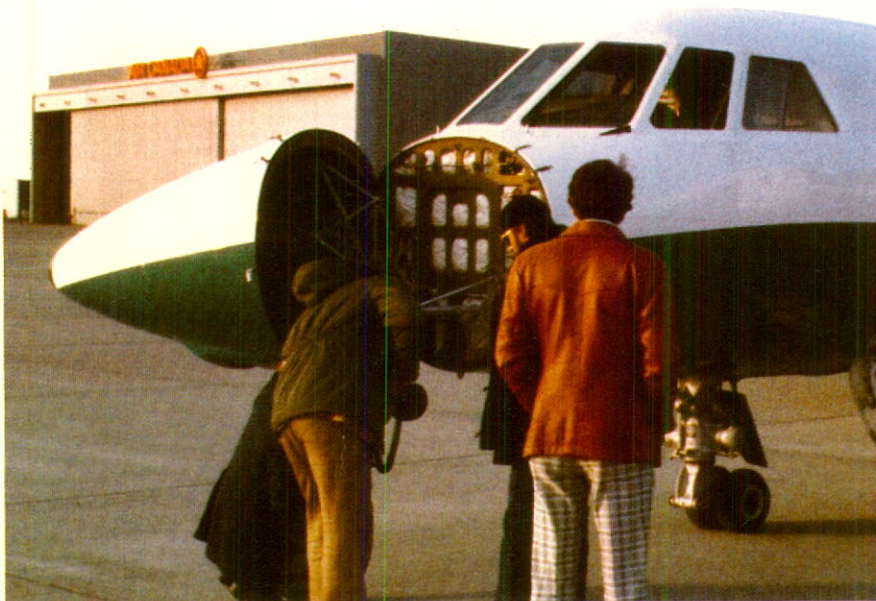
Specially equipped aircraft used for aerial thermographic survey.
