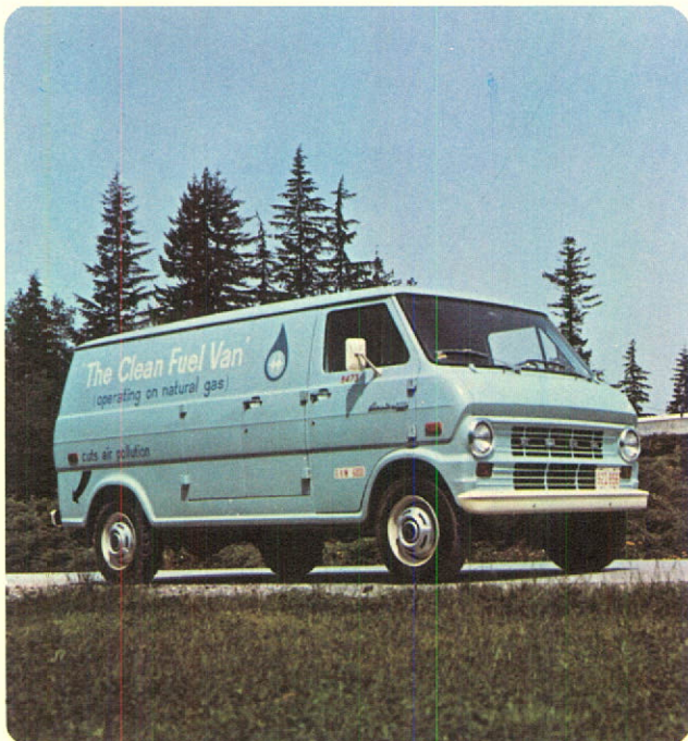
B.C. Hydro's natural gas-fuelled van reduces air pollution.
