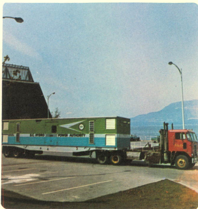
Mobile diesel generating units supply power in some areas that are not connected to the integrated electric system.
