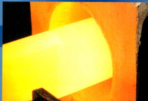
Heat treating A-312 pipe
