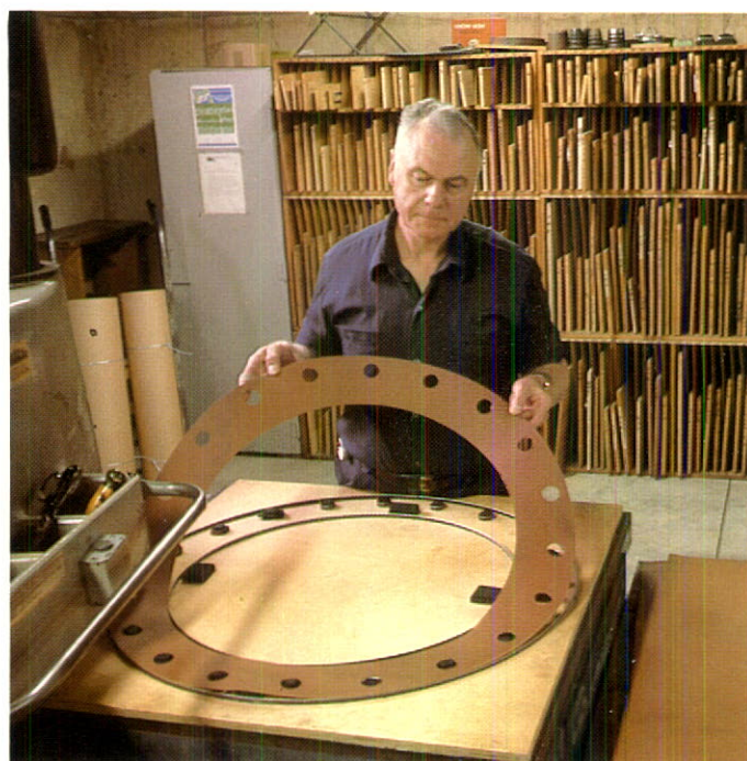
Sid Dixon removes a gasket, just cut out of Goodyear's red rubber, at Snowden Rubber Industries in Oshawa, Ontario.
