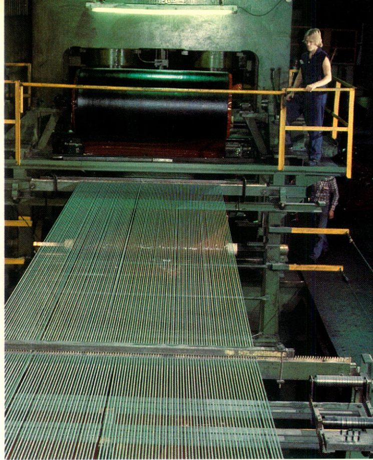
Strands of steel cable are drawn in conveyor belt compacter at Bowmanville plant, prior to curing (above). The steel-cable belting is destined for use at oil sands projects in Northern Alberta.
