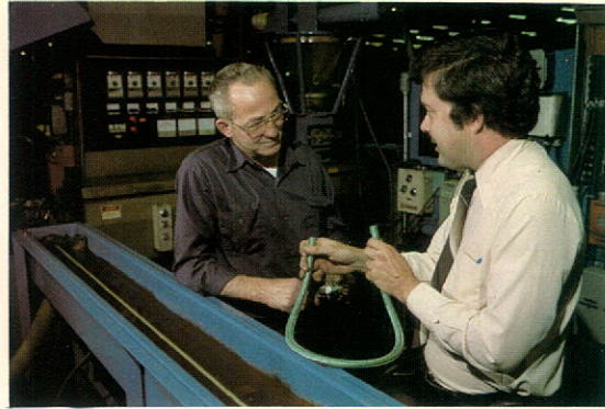
The development of thermoplastic hose for industrial and farm applications was a top priority in 1982. Terry Jackson, development manager and machine operator Bill Kennedy examine a sample of plastic hose inner liner at extrusion stage of production (above).
