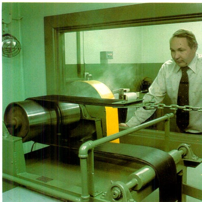
Shown here undergoing a severe friction test, 'Pylon II' meets all government specifications for underground mining applications. Lindsay Terreau, the plant's chief chemist looks on.
