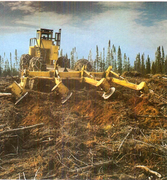
Tilling or scarifying the soil on a cutover forest site in preparation for planting or seeding is a key step in the regeneration process. The above powered-head scarifier, designed and developed by our woodlands personnel and Northern Engineering & Supply Co. Ltd. of Thunder Bay, is proving adaptable to the rugged terrain of Northwestern Ontario and provides higher productivity than other types of scarifying equipment.
