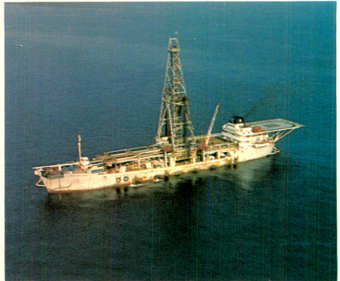
The Glomar Grand Banks drill ship commenced drilling the Vega No. 1 well in August 1980. The location is in 413 ft. of water and has a projected total depth of 15,750 ft.
