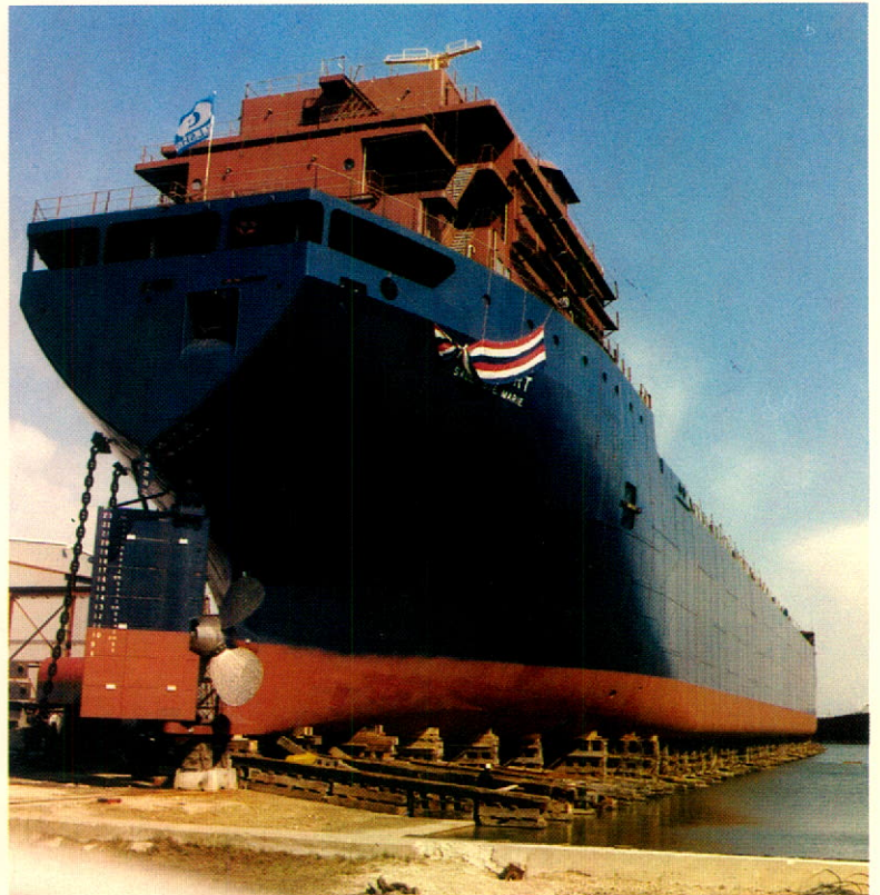
Immediately before launching the vessel has been raised from the "keel blocks" to the "ways".
