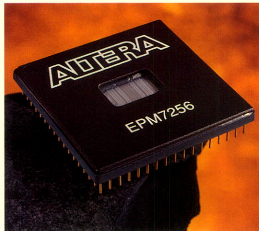
The EPM7256 MAX EPLD offers up to 10,000 gates and the highest pin-to-gate ratio available in the industry today.
