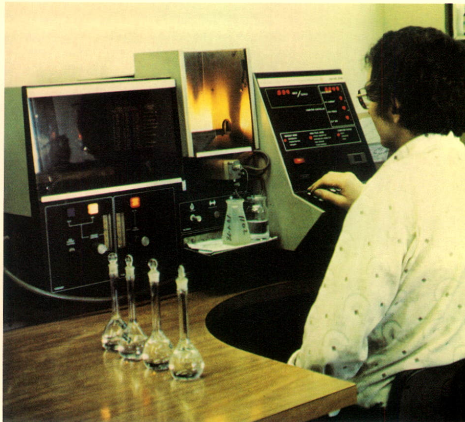
Ore and concentrates assaying with spectrographic analyzer
