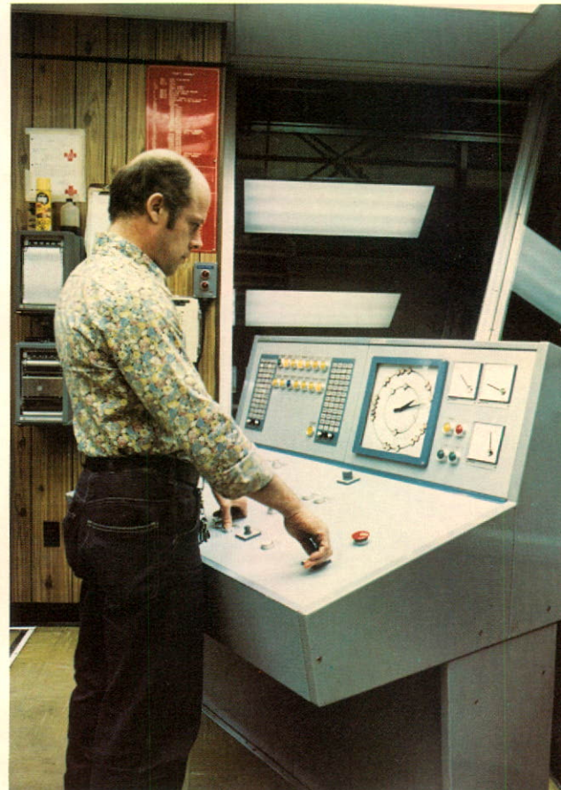
Hoistman at controls — No. 12 Mine, No. 2 Shaft, 3100 ft.
