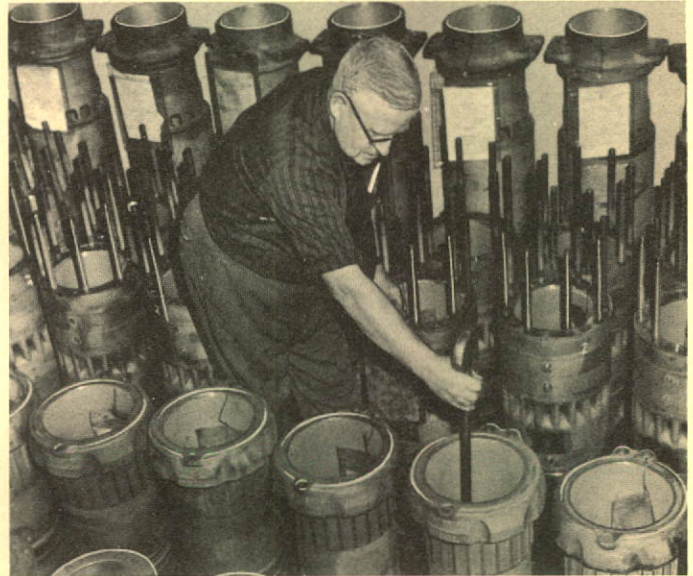
Besides making slotted, conically drilled and perforated screen plates used in screening operations by the pulp industry, The Union Screen Plate Company of Canada (Limited) operates the largest industrial plating facility in Canada. Among the services performed by this subsidiary are plating operations for the railways and the marine and pulp industries. The photo shows measurements being taken on chrome plated railway diesel cylinders which have been re-lined to outlast the original finish.
