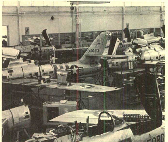
One of the largest civil and military airplane repair and overhaul organizations in Canada, Northwest Industries Limited is currently working on a contract for the inspection, repair and overhaul of F-84 jet fighters for the U.S. Air Force. The total number involved is 112, of which 60 have been completed. Some of the airplanes were transported to Canada from the Orient by aircraft carrier, and others were flown to Edmonton from bases in the United States.
