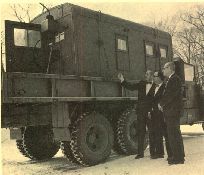
Oneida Electronics Inc., the CAE subsidiary in Utica, N.Y., is in the final stages of work on a contract for the manufacture of 229 field radio-teletype systems for the U.S. Army Signal Corps. To date 210 of the units have been completed. They are mobile receiving and transmitting stations which will receive radio messages and relay them in teletype form, or receive teletype messages and pass them on as radio impulses. One is shown above ready for shipment.
