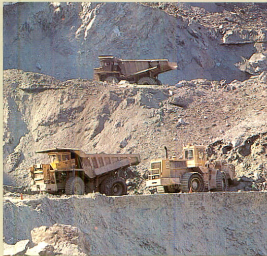
50 to 70 ton capacity off-highway trucks are used to haul ore from the pit.
