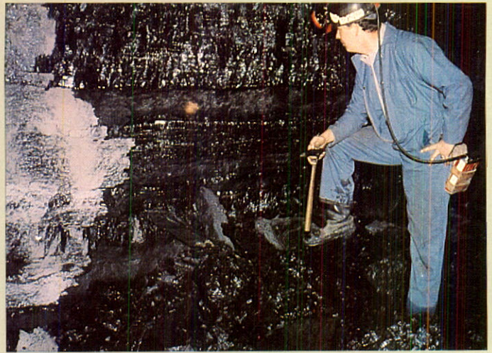
Buddy Hall, Mine Superintendent of Loftis Coal Division examining 60 inch seam underground. Clean coal thickness in the seam is 45".
