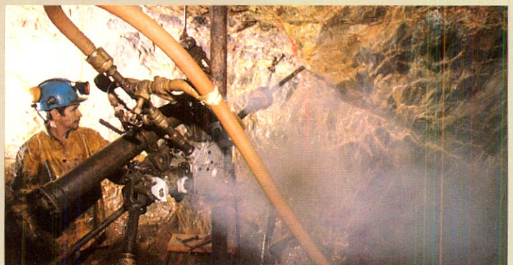
Diamond drill working on the twelfth level as part of a 6000 foot drilling program.
