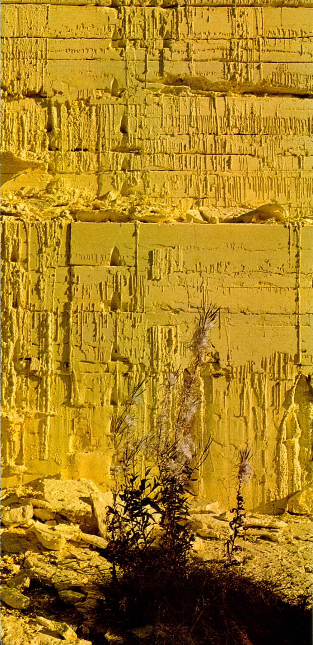
Massive block of sulphur removed from sour natural gas at the Fort Nelson sulphur recovery plant. The sulphur is poured when molten into movable aluminum forms which shape it into blocks. Substantial tonnages have been stored at Fort Nelson for two years due to weak market prices. A recent strengthening in price suggests it may soon become economically practical to transport it to outside markets.
