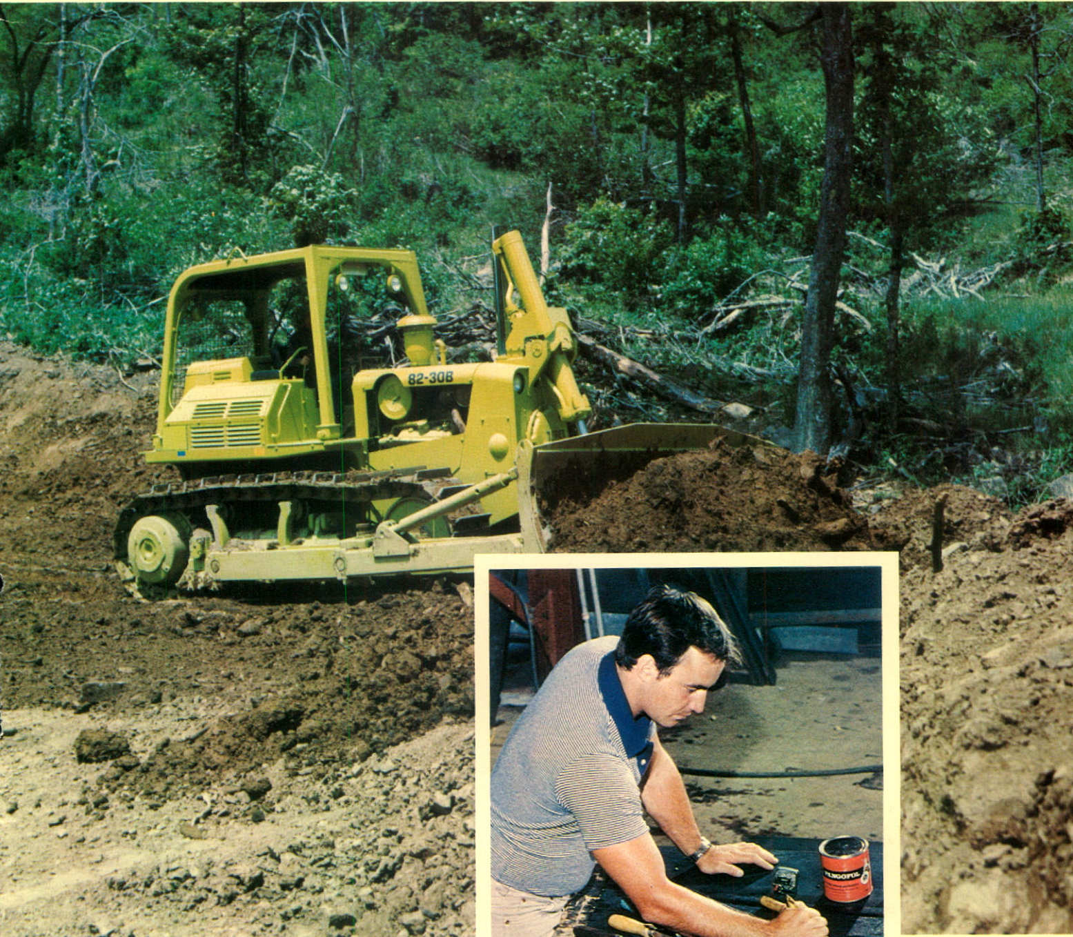
(Large photo) Terex-IBH model 82-30B, 275 h.p. crawler tractor. Used widely in construction and forestry applications.
