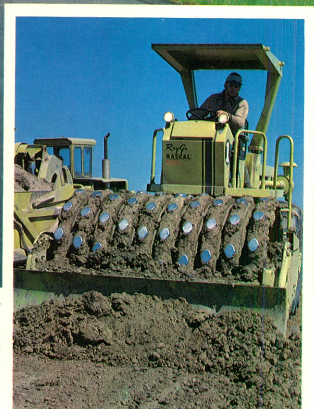
(Large photo) RayGo Ranger 2-66 compactor. Rolling asphalt on a provincial highway near Daulphin, Manitoba.
