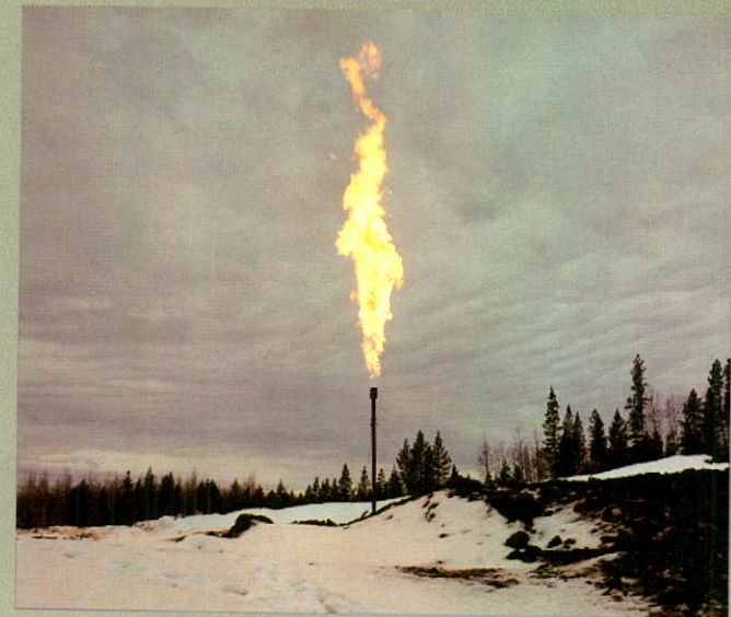
Flow testing Canadian-Hunter Bluesky et al well in the Elmworth area of western Alberta.
