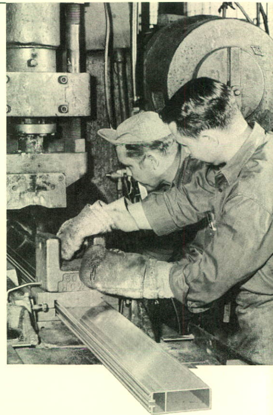
This press extrudes structural shapes from aluminum billets under a pressure of 4,000,000 pounds.
