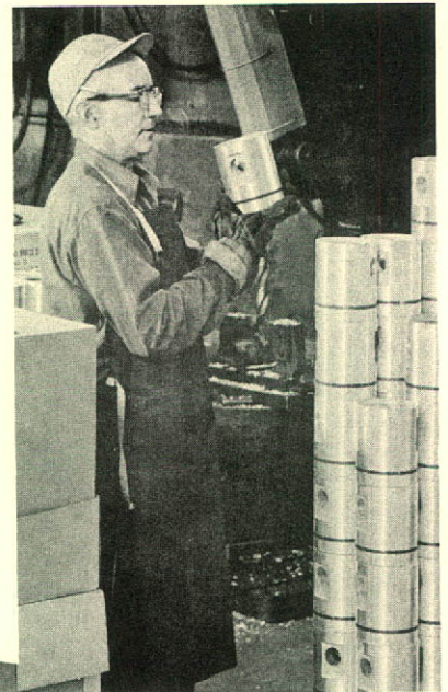
Packaging for shipment—Bohn aluminum pistons for heavy-duty diesel engines used in earth-moving road construction.
