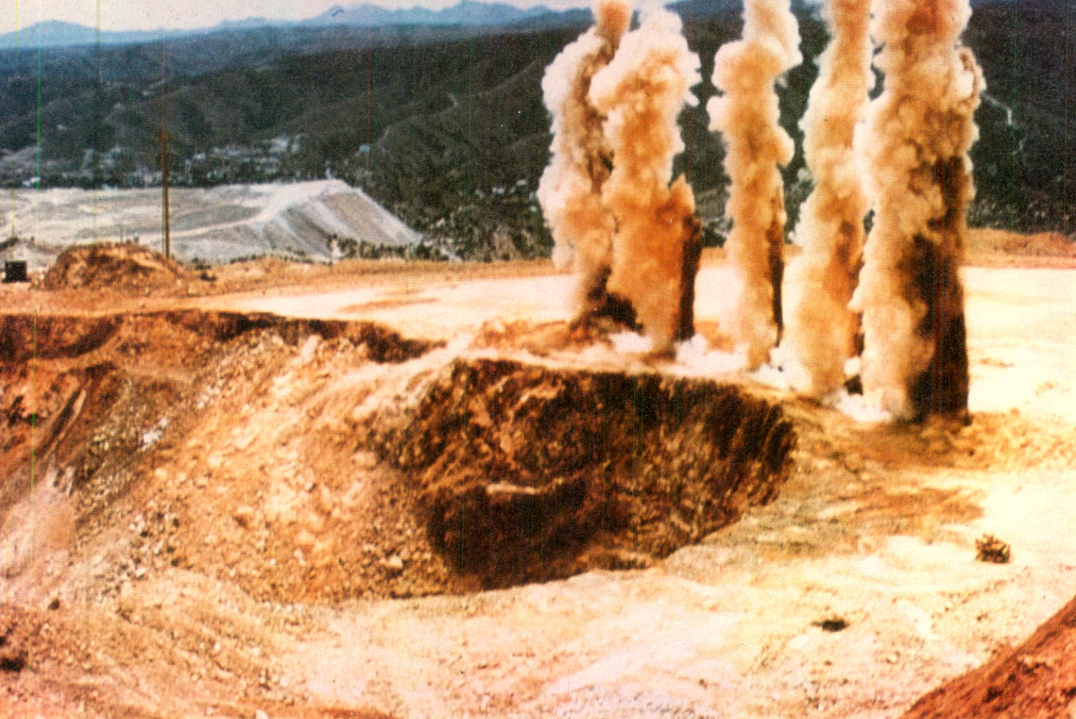
A five-charge blast breaks copper ore at one of Inspiration Consolidated Copper's many open-pit mines in Arizona
