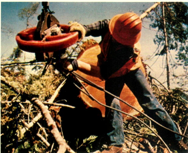
Timber is felled, bucked and lifted out by helicopter to "waterdrop" landing areas where it is processed, boomed and towed to the sawmill.
