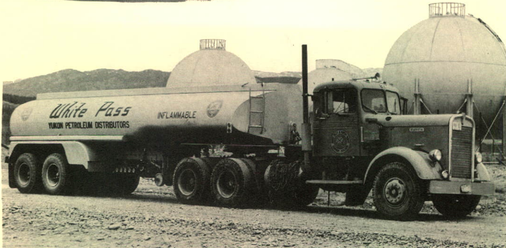
Tanker-trailer unit used in delivering petroleum products to Highway points — spherical storage tanks in background.
