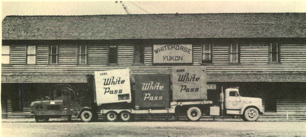
Steel cargo containers loaded on flat bed truck for delivery to consignee at Whitehorse—Company railway station in background.
