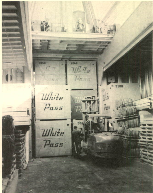
Stowing steel cargo containers in hold of M.V. "Clifford J. Rogers". Vessel is designed to accommodate 168 containers.
