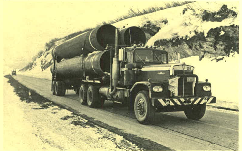
One of the Company's trucks hauling 48" diameter pipe from Valdez to Fairbanks for the proposed oil pipeline from the North Slope of Alaska to Valdez.
