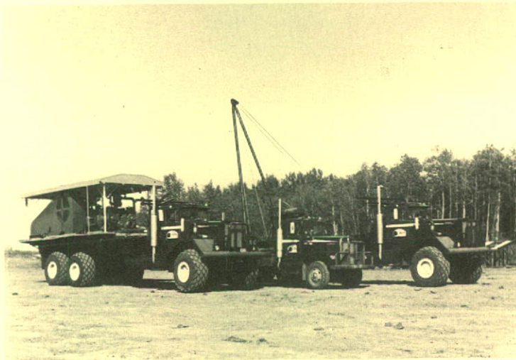
Two specially designed and equipped model 953 Kenworth trucks dwarf a conventional model 924 Kenworth truck. These large units are capable of carrying a payload of 50 tons, are all wheel planetary drive and are equipped with special flotation tires to reduce ground pressure in tundra areas.
