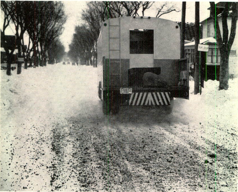
Cinder spreader designed and built by Company employees.
