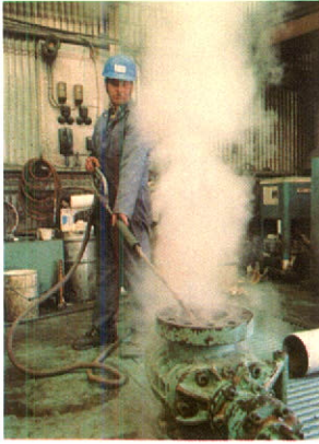
Cleaning a rental well blow-out preventer prior to painting.
