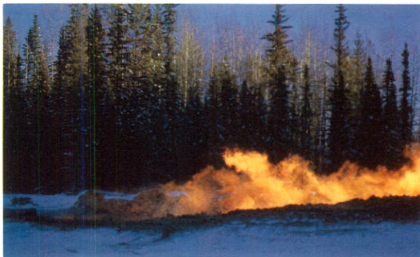
Flow testing on completion off Sikanni Well.
