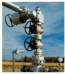
A producing well is identified by this wellhead device called a "christmas tree".
