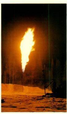
A brief flow and flame test is used to evaluate potential production at a natural gas discovery well.
