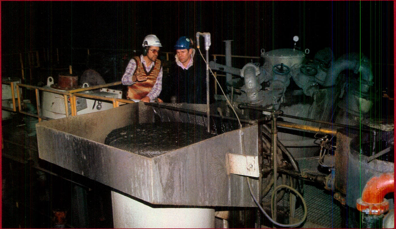
In response to poor base metal markets skilled people within the Placer group are finding better and cheaper methods to mine and mill ore. At the Gibraltar open pit copper mine in British Columbia's Cariboo region, column flotation technology, first used in the petro-chemical industry, is being tested with the objective of reducing concentrator operating costs and improving metal recovery. Mine Manager Jeff Thompson (right) examines column with Project Engineer Roger Amelunxen.
