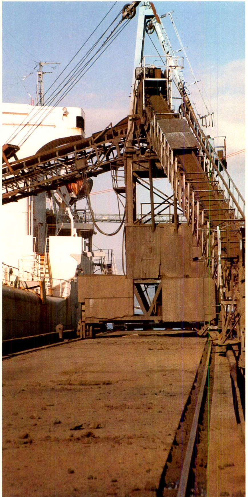
Copper concentrate is loaded aboard deepsea bulk carrier for transport to Japan where it will be smelted and refined into pure copper.
