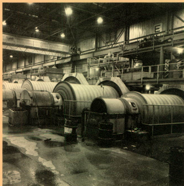
New technologies allow processing of large quantities of ore in concentrators such as this at Gibraltar copper mine, opened in 1972.
