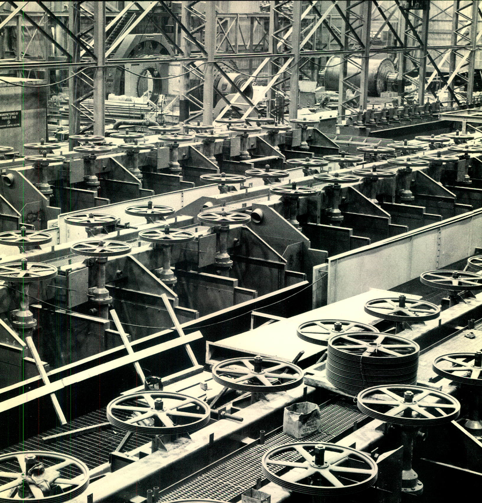
View over rows of flotation cells in concentrator shows grinding mills in background.
