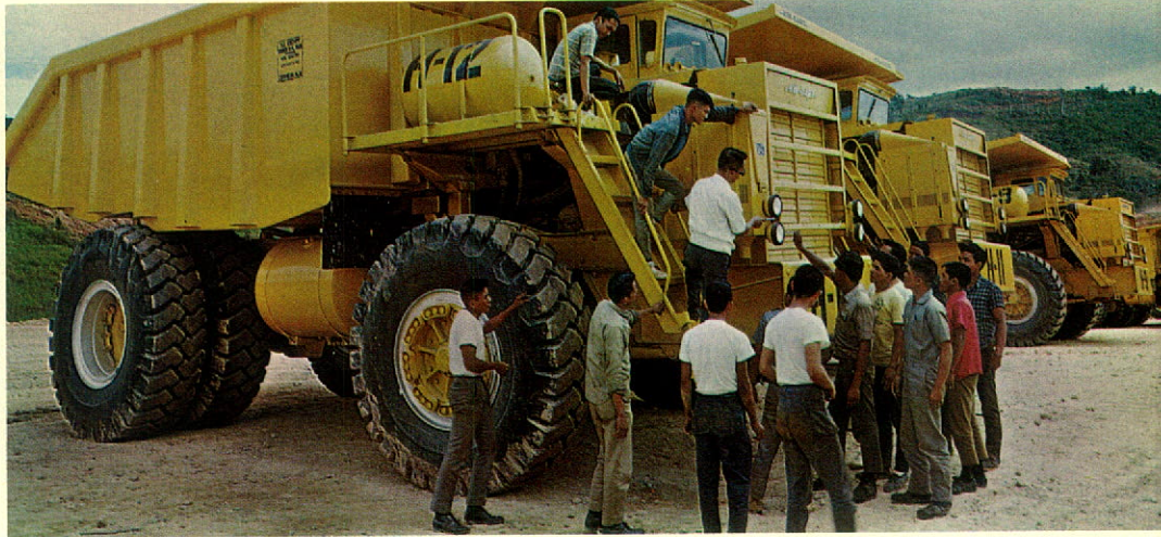
In anticipation of the start of Marcopper's production, apprentices receive instruction on the care and maintenance of 75 ton pit haulage trucks.
