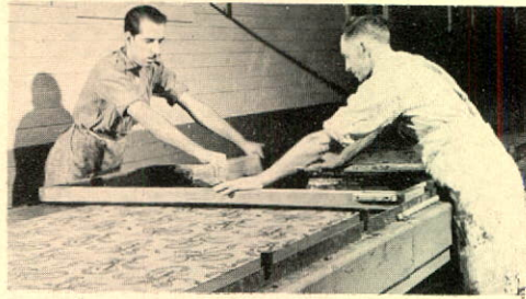
Hand screen printing. Patterns are stencilled on cloth which is affixed to 70 yard tables.
