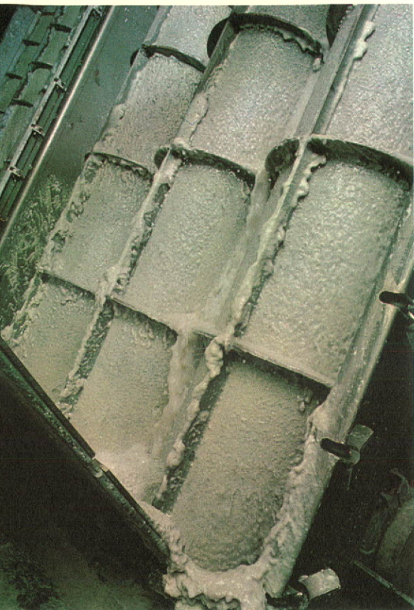
Screw extractors (above) remove ink from wastepaper at the secondary fibre pulp mill.
