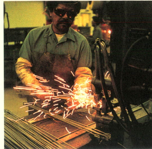
Loop ties are being welded at the Symons plant. These ties are used to hold Steel-Ply® forms together to make walls into which concrete is poured for forming concrete.
