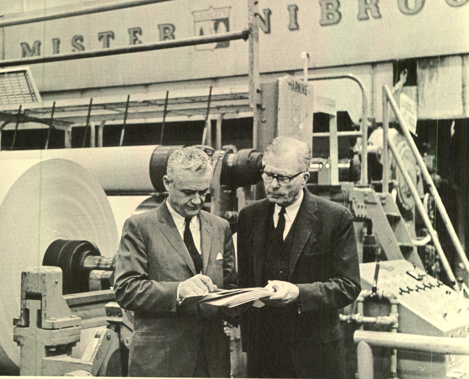
Chairman of the Board William L. Keady (right), and President Leonard A. Pierce discuss sheet formation of creped kraft towel paper made on the 196" paper machine in background. This machine, located at the Cascade paper mill in Gorham, N.H., produces a mile of towel paper fifteen feet wide every four minutes.
