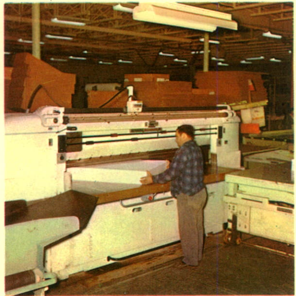
This modern, fully-automatic paper trimmer is one of the largest and most accurate in the industry. This machine spaces itself automatically, thus eliminating the human error in cutting sheets to size.
