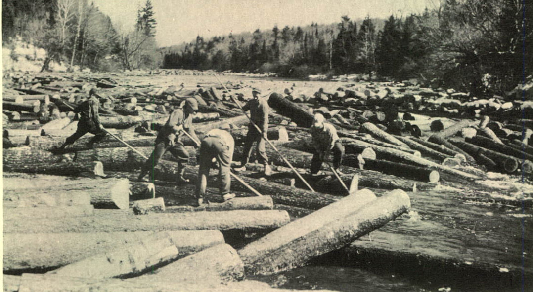
Softwood logs on their way to the sawmills at Berlin are freed by these expert river drivers on the Androscoggin River. Transportation by water gives substantial savings as compared with trucking.
