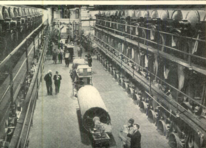
Visitors are dwarfed by these sulphite pulp dryers, which turn out high-quality pulps for use in cellophane, writing papers, photographic papers, and many other items.
