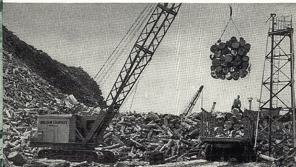
▲ Four-foot pulpwood is efficiently unloaded from trucks at Berlin, N. H., by the use of a special sling which enables each tier of wood to be unloaded in one lift by the crane. When the sling-load strikes the pulpwood pile it is immediately released. Other cranes, visible in the distance, work on the same pile.
