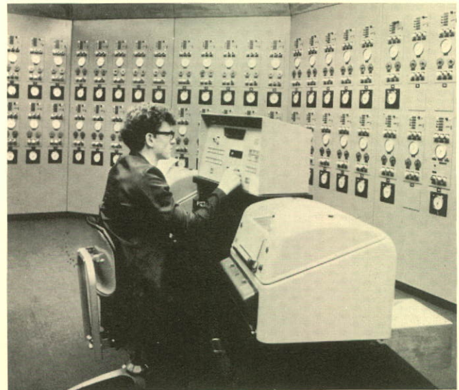
One of the most significant installations during 1969 was the computerized dye-house. This photo shows the central control room where more than 60 dyeing machines can be monitored.
