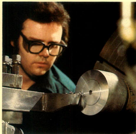
A welder in the Edmonton shop puts the finishing face on a lead impression block.
