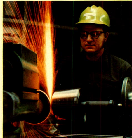
The face of an A.P.I. plug gage for rotary connections is precision ground to close tolerances on a tool and cutter grinder by Tommy Parrish.
