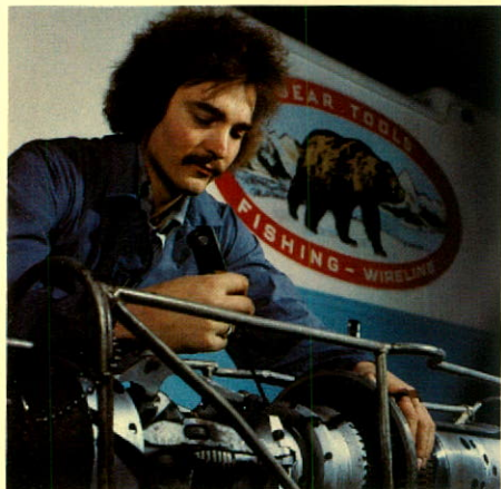
Larry Hoblack, wire line operator, servicing a 9 5/8" dia-log caliper tool used for inspecting the general condition of down-hole casing.
