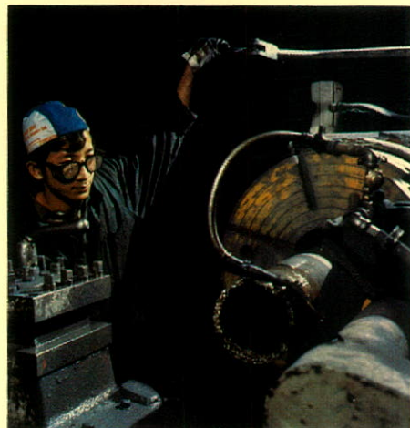
Nhi Nguyen, welder, grinds the O.D. of a wash-over shoe to the specific size required for a job.
