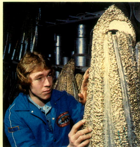
Allan Bellinger, Edmonton head shop hand, inspects a tapered sinter cut mill, used for milling through collapsed sections of casing down the hole.
