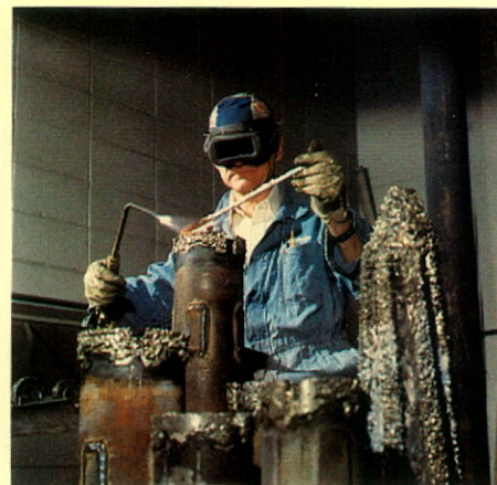
George Ullman, chief welder, applies tungsten carbide chips to the face of a wash-over shoe.
