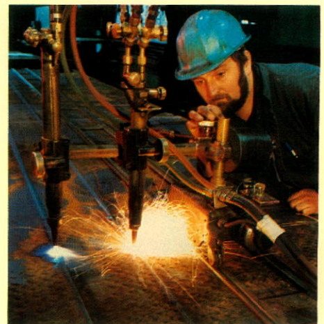
Detail of heavy gauge steel plate being cut into measured strips.
