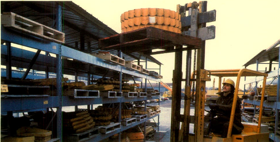
Weather-tolerant large castings placed by an Allis-Chalmers fork lift truck in an extensive outdoor storage facility.
